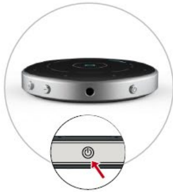
Power On Table Microphone Streaming starts in hearing aids automatically
